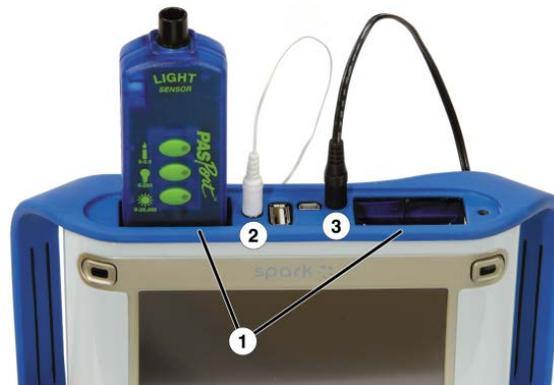
Figure 1: SPARK SLS showing the location of the PASPORT ports (1)
